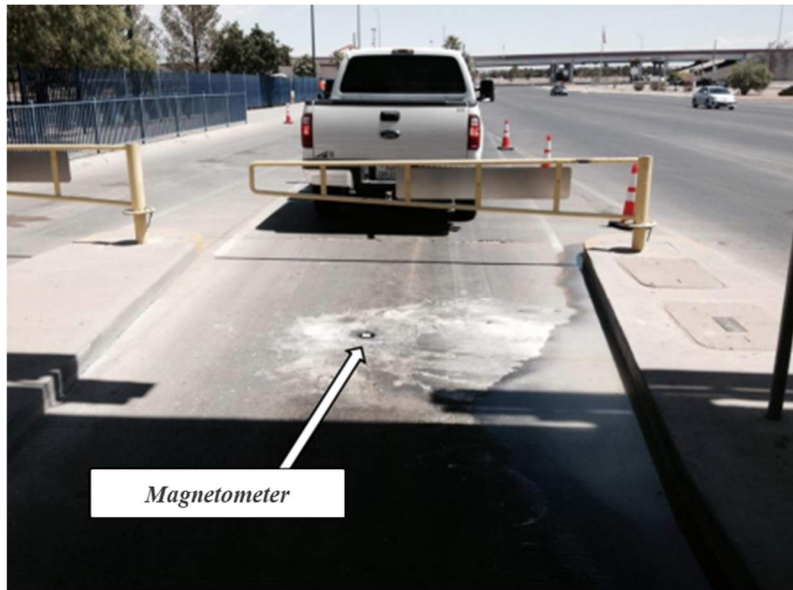
Figure 13. Magnetometer Technology Testing at a Border Crossing 8
