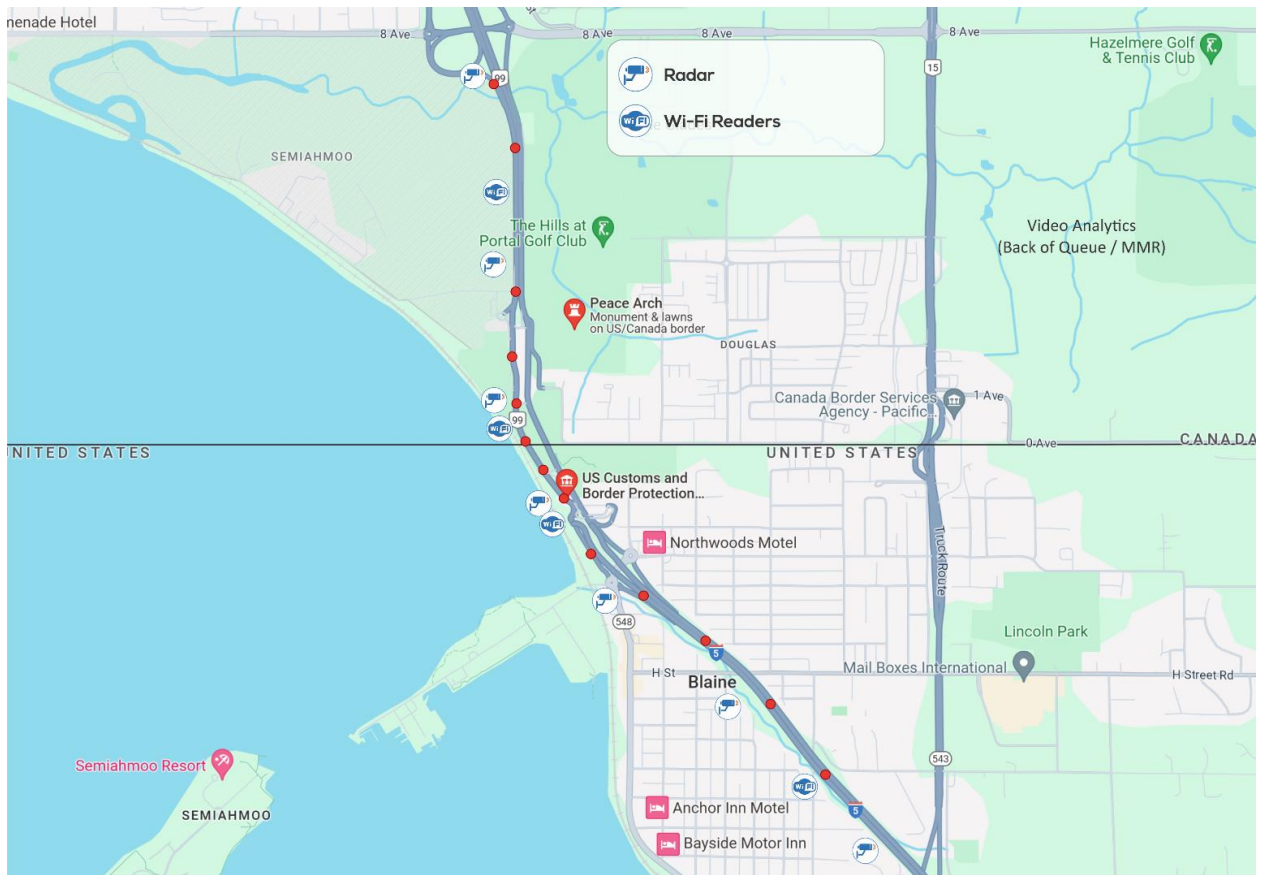
Figure 10. Proposed Roadside BWT Measurement Technologies
