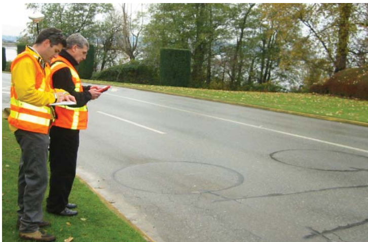
Figure 4: Collecting GPS Data for Loop Detectors
